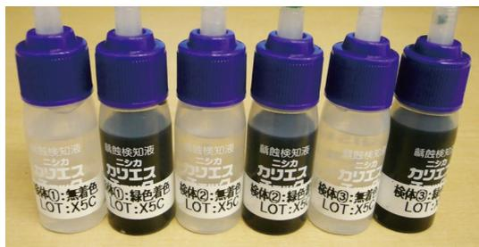
**Fig. 1** The experimental caries-detecting dye solution containing high laser-absorptive substances (urea)
