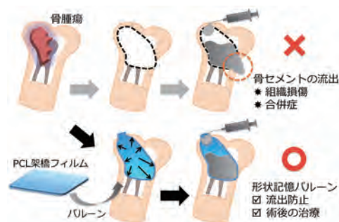
Figure 1. Schematic illustration of PCL balloon system for bone tumor treatment.
