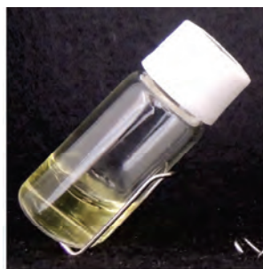
Fig. 1 Acrylamide gel containing DTB-PAS-DA as a cross-linker
